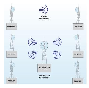
This transmitter can be used to feed a single link or several links simultaneously. A typical application example would be a single 6-mile (10-kilometer) link with 40 channel loading, or four simultaneous links of 3 miles (5 kilometers) each.
