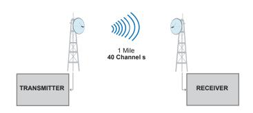
A typical application example would be a one-mile (1.6-kilometers) link with 40 channel loading.
