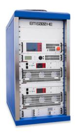
The 7.5KW FM transmitter **EM 7500 HE HOT PLUG** has been created for high efficiency transmitters with hot plug modules. It consists on four FMA 2000 HE power amplifiers with >73% efficiency (they can be externally used as 2KW amplifiers) and the EM 100 DIG PLUS transmitter. This high efficiency 7.5KW amplifier has an approximate consumption of <11KVA, so it pays for itself in a short period of time due to its low consumption. This transmitter can be supplied with the following options:
