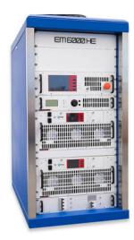
The 6KW FM transmitter **EM 6000 HE DIG PLUS** has been created for high efficiency transmitters. It consists on the FMA 6000 HE power amplifier with >73% efficiency and the EM 100 DIG PLUS transmitter. This high efficiency 6KW amplifier is composed by two 3-3.5KW amplifying units (FMA 3000 HE) and it has an approximate consumption of 8600VA at 230Vac, so it pays for itself in a short period of time due to its low consumption. This transmitter can be supplied with the following options:
