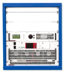
The **3.5KW FM transmitter EM 3500 HE DIG PLUS** has been created for high efficiency transmitters. It consists on the FMA 3500 HE power amplifier with >73% efficiency and the **EM 25 DIG PLUS transmitter**. This high efficiency 3.5KW amplifier has an approximate consumption of 4900VA at 230Vac, so it pays for itself in a short period of time due to its low consumption. This transmitter can be supplied with the following options:
