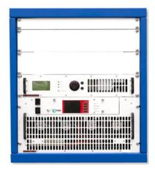
The **3KW FM transmitter EM 3000 HE DIG PLUS** has been created for high efficiency transmitters. It consists on the FMA 3000 HE power amplifier with >73% efficiency and the EM 25 DIG PLUS transmitter. This high efficiency 3KW amplifier has an approximate consumption of 4200VA at 230Vac, so it pays for itself in a short period of time due to its low consumption. This transmitter can be supplied with the following options:
