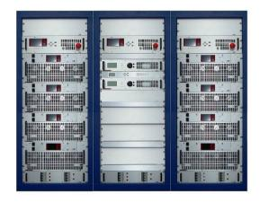
The **25KW FM transmitter EM 25000 HE DIG PLUS** has been created for high efficiency transmitters. It consists on the FMA 25000 HE power amplifier and the EM 250 DIG PLUS transmitter. This high efficiency 25KW amplifier is composed by eight 3.5KW amplifying units (FMA 3500 HE). This transmitter can be supplied with the following options:
