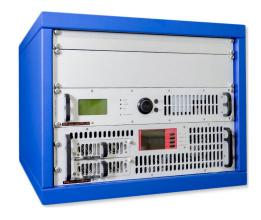
The 2KW FM transmitter **EM 2000 HE DIG PLUS HPPS** has been created for high efficiency transmitters. It consists on the FMA 2000 HE HPPS power amplifier with >73% efficiency and the **EM 25 DIG PLUS transmitter**. This high efficiency 2KW amplifier has an approximate consumption of 2600VA at 230Vac, so it pays for itself in a short period of time due to its low consumption. This transmitter can be supplied with the following options:
