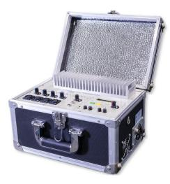
The **portable FM transmitter MRI 15 DIG** is specially designed for the following applications: Civil Defense, Armed and security Forces, electoral campaigns, religious orders, small communities, etc. This portable transmitter MRI 15 DIG is composed by a four audiochannel mixer and an externally synthesized 15W FM transmitter with RF output signal. It has been designed to work as an emergency radio station, easy to use and to install.
