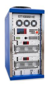
The **10KW FM transmitter EM 10000 HE DIG PLUS** has been created for high efficiency transmitters. It consists on the FMA 10000 HE power amplifier with >70% efficiency and the EM 100 DIG PLUS transmitter. This high efficiency 10KW amplifier is composed by two 5KW amplifying units (FMA 5000 HE) and it has an approximate consumption of 14.2kVA, so it pays for itself in a short period of time due to its low consumption. This transmitter can be supplied with the following options:
